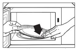
The turntable can be removed for cleaning. Always keep the roller ring underneath it clean as well as the oven floor. Otherwise the ring might not run smoothly.
